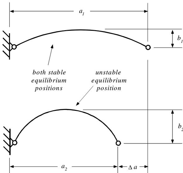
**Figure 18: Determination of horizontal and vertical deflections**
