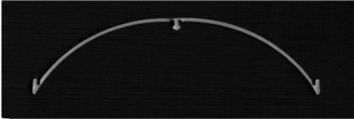
Figure 14: Bistable CD ejection actuator
