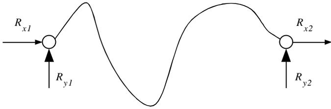
Figure 1: A general functionally binary pinned-pinned (FBPP) segment
