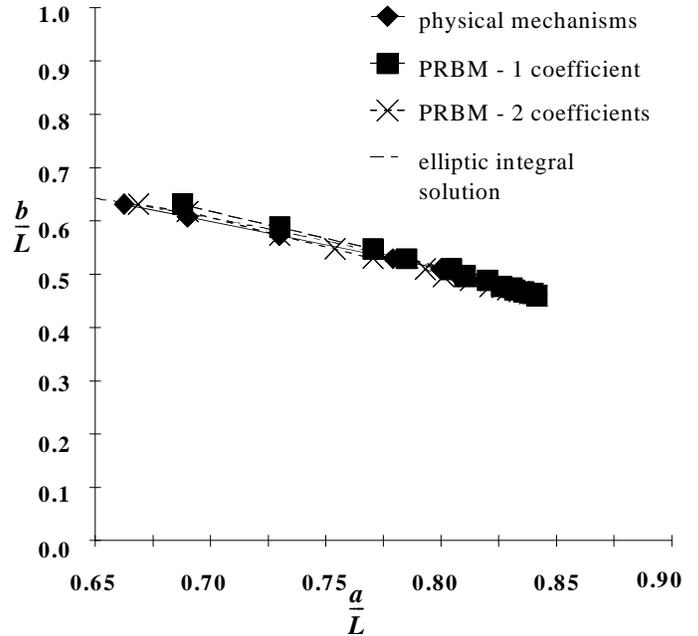
**Figure 12: Aluminum deflection path for  $\kappa_0 = 1.0$**
